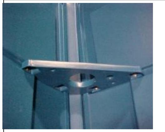
17. Insert vent tube through roof and shelf into the tank recess. (see Fig. A) Using a 3/16" Drill Bit Drill hole at location shown (see Fig. B). Fasten with Rivet, Silver Long #18755 (1).
