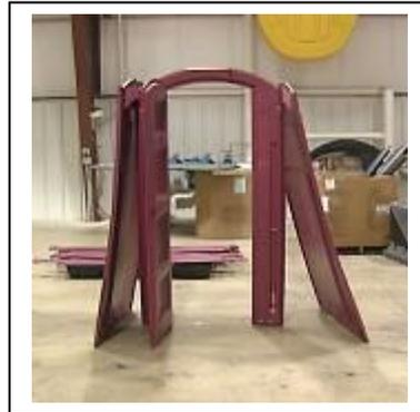
5. Rivet right panel to door jamb- fasten top, center and bottom using Rivet Expanding #18755 (32) and repeat on left side. This will hold parts together. (Note: The panels overlap on the front. Also you can finish riveting remaining holes at this time.)
