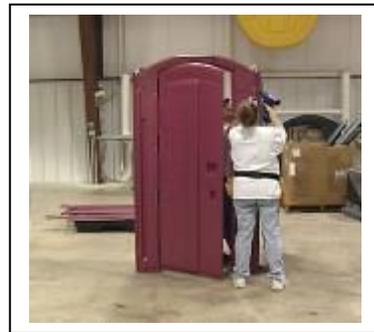
6. Fasten the right wall, back wall and post together. Rivet the top hole with Rivet Expanding #18755 first. Then finish riveting remaining holes with Rivet Expanding #18755 (32). Repeat the same step on the left side. (Note: The rear panel needs to overlap the left side panel and the right side panel needs to overlap the rear panel on the rear of the toilet.)
