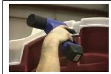
10. Fasten the tank to the back wall. Drill 1/4" hole through each tank tab and back wall. Fasten the tank to the back wall with 1/4-20 x 3/4 Truss STNLS #18705 (2), Nut, 1/4-20 nylon #13128 (2) and Washer, 1/4" flat #12382 (2). Washers and nuts are on the outside of the unit.
