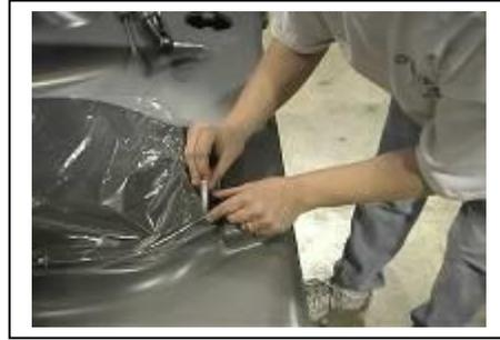
3. Remove shipping screw from bottom of door and open door to 90 degrees.
